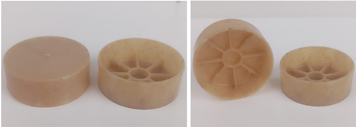
Figure 20 Trial 3 samples containing 100% recycled CO189.
