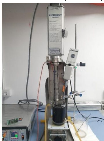
Figure 10: Ultrasonic probe setup.
