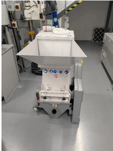
Figure 5: Piovan G17-38 granulator used to mechanically downsize the panels at NCC.
