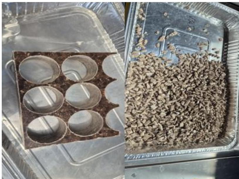
Figure 23: Left: Machined wood composite test plate; Right: The granulated wood composite. The maximum particle size is 10 mm.
