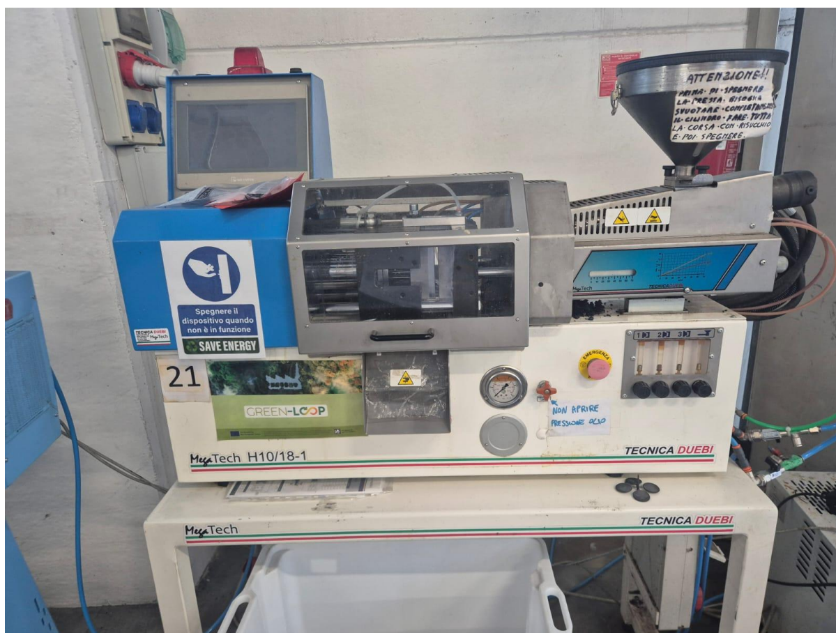
Figure 17: Lab-scale Megatech H10/18-1 machine.
