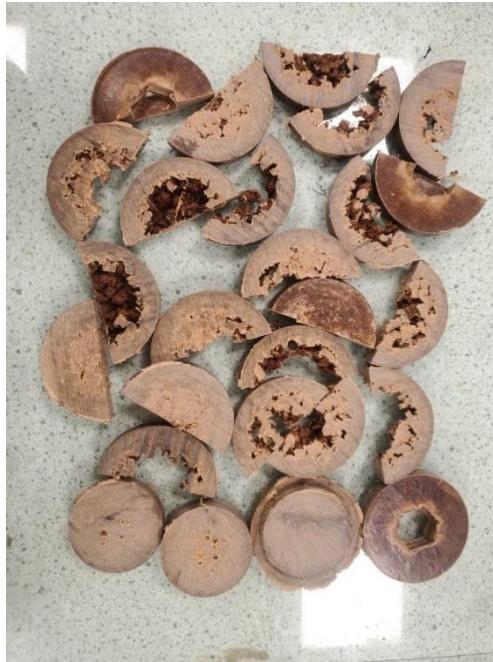
Figure 21: Wood composite offcuts, cut down to 1cm thick strips prior to granulation.
