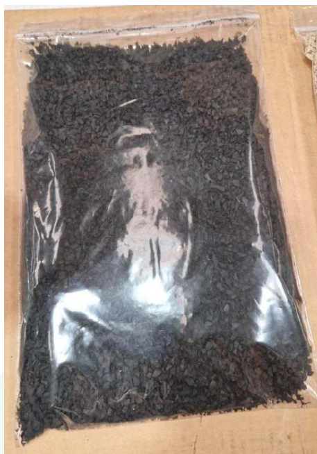
Figure 8: The final rubber granulate prior to reprocessing.
