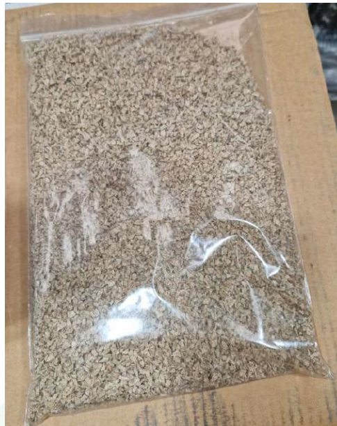
Figure 22: The granulated wood composite. The maximum particle size is 5mm.
