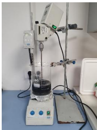
Figure 9: Overhead stirrer and heater used to mix the rubber and oil.
