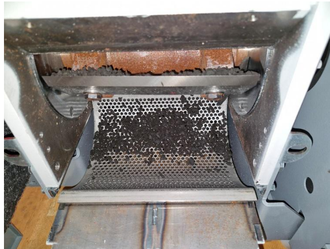
Figure 7: Rubber granules contained within the granulator. The crumb size is controlled by the hole size within the grate.
