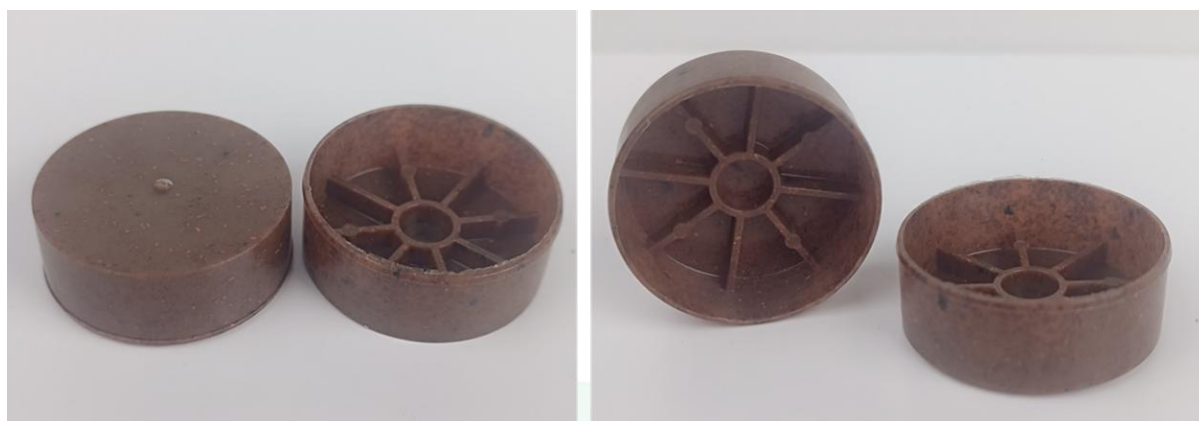
Figure 19: Trial 2 samples containing 15% recycled mix of CO220/T23088/T23090.
