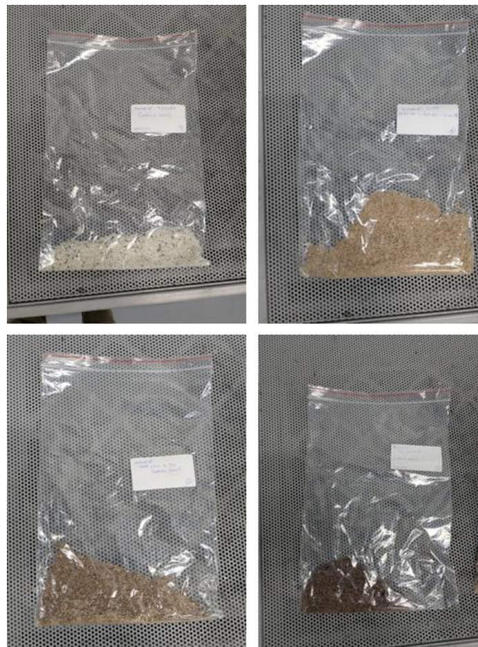
Figure 16: Four types of bottle closure were granulated. The maximum particle size is 5mm.
