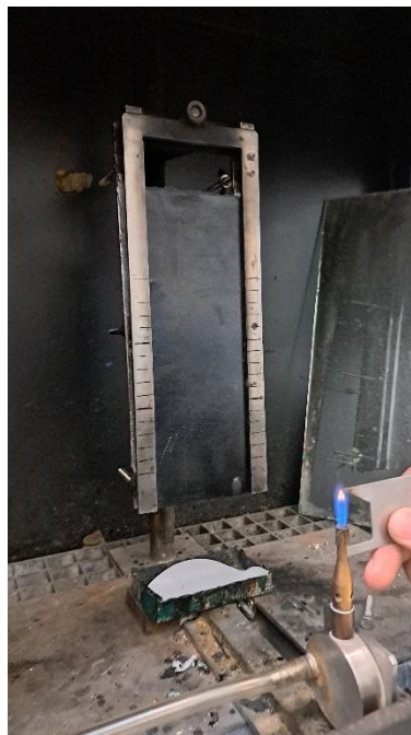
Figure 6: test specimen and pilot flame, calibrated before the test.
