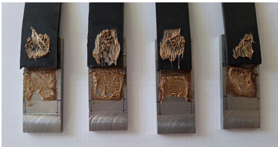
Figure 53: Failure modes of GL-P-017A bio rubber after adhesion test.
