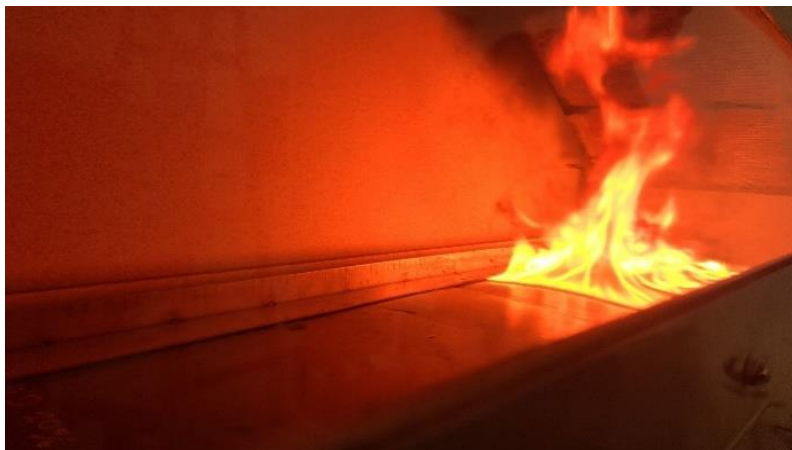
Figure 16: Ignition of the rubber after pilot flame exposure at one end of the specimen.
