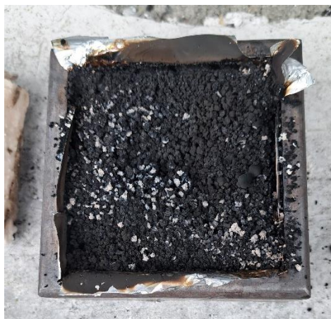
Figure 21: samples for ISO 5660-1 test after the testing.
