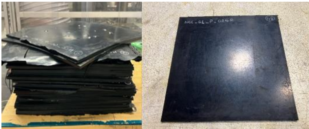
Figure 3: Rubber panels produced with dimensions of 500 x 500 x 10 mm.
