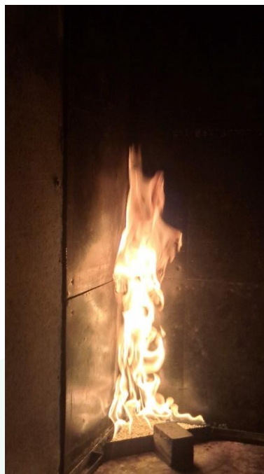
Figure 10: Test specimen at the beginning of the test after ignition of the burner, but before tested material ignited.
