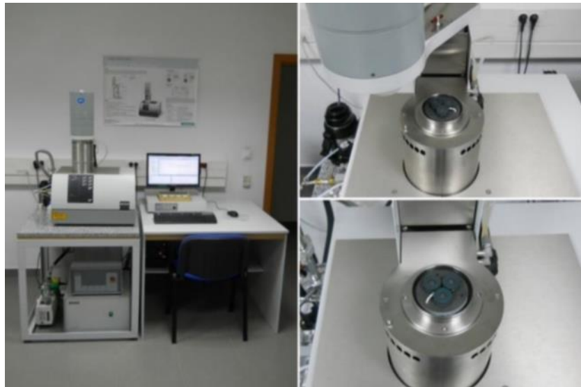
Figure 34: Netzsch LFA 457 thermal test equipment
