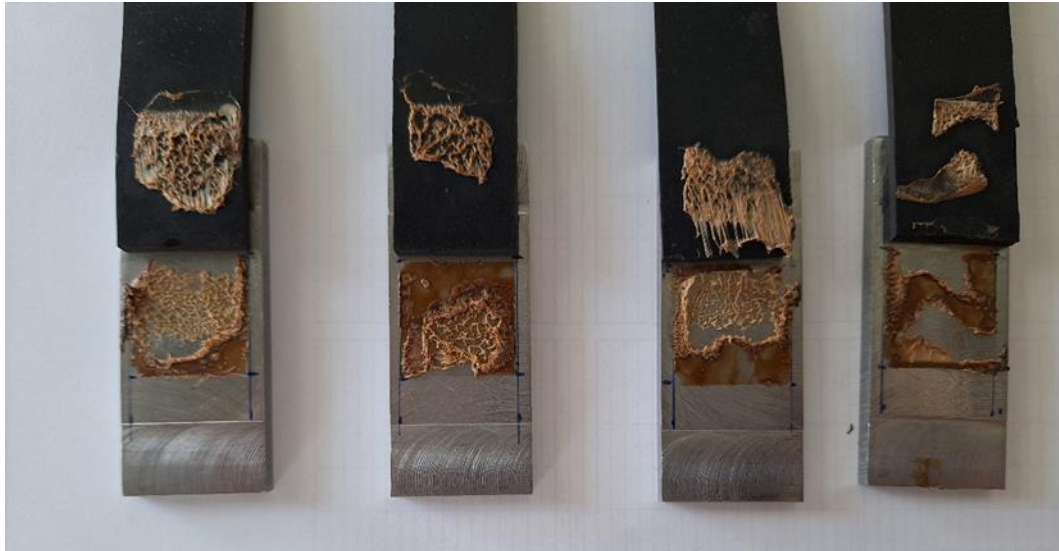
Figure 52: Failure modes of GL-P-018B bio rubber after adhesion test.
