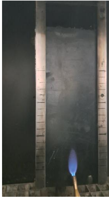
Figure 7: test specimen during the test with surface exposed to the pilot flame.
