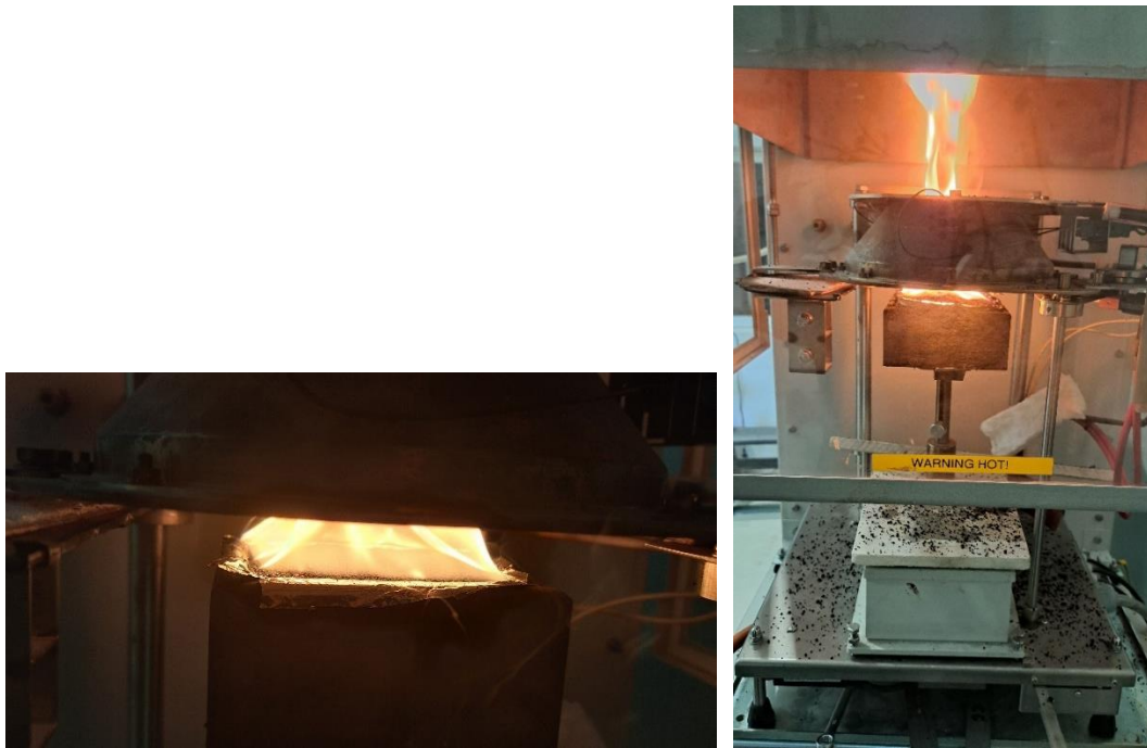
Figure 20: samples for ISO 5660-1 test during the testing.
