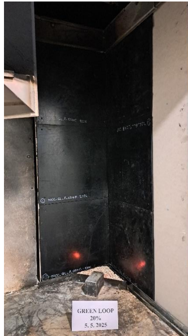
Figure 9: Test specimen before start of the SBI test.
