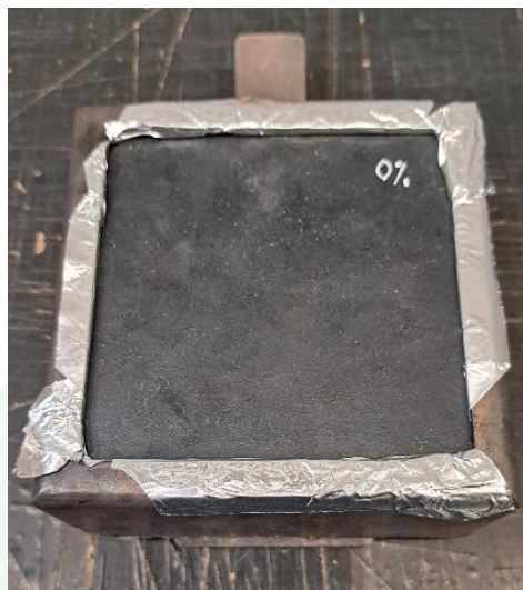
Figure 18: samples for ISO 5660-1 test prior the testing.
