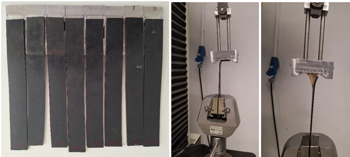
Figure 49: Specimens of bio rubber used for the adhesion test
