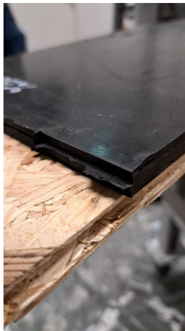
Figure 14: Product was placed on the wooden substrate (OSB).
