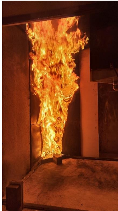
Figure 11: Burning test specimen after 10 minutes of testing time, before the test need to be stopped from safety reasons.
