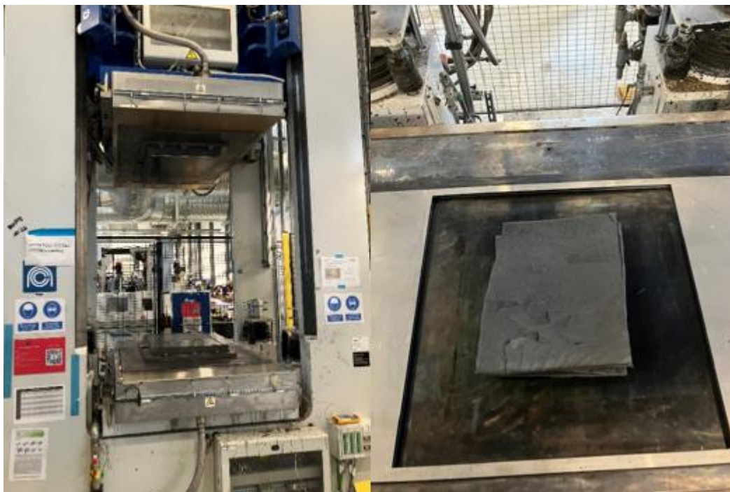
Figure 2: (Left) 1100 tonne hydraulic press, (right) material loaded into tool prior to pressing.
