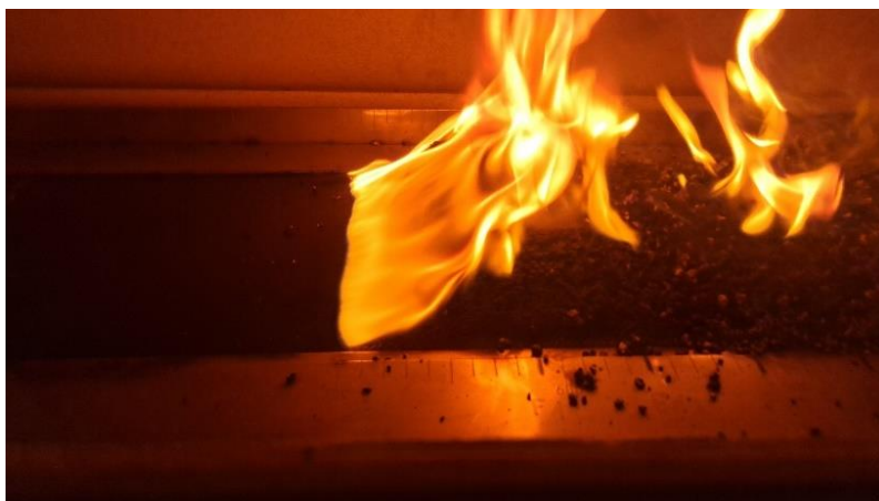
Figure 17: Propagation of fire front during the test.
