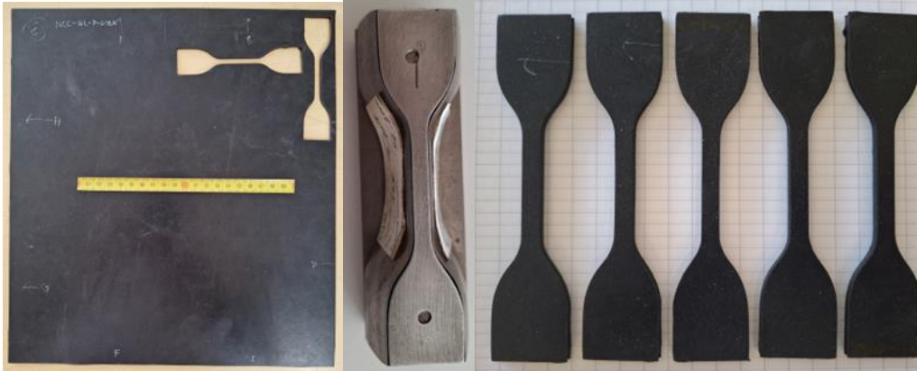
Figure 55: Left to right, bio rubber pad after some specimens extracted, specimen cutting tool and test specimens ready.
