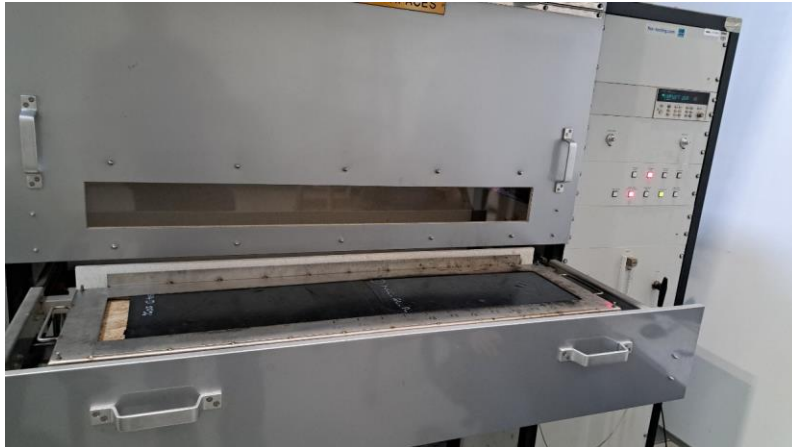
Figure 15: Test apparatus with test specimen before exposure to heat flux.
