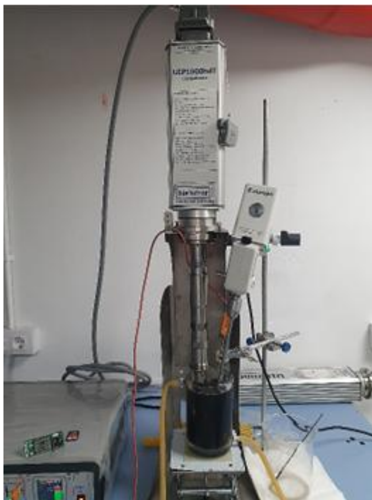
Figure 9. Ultrasound assisted chemical devulcanization of rubber crumb with 2 kW prototype at IRIS facilities.
