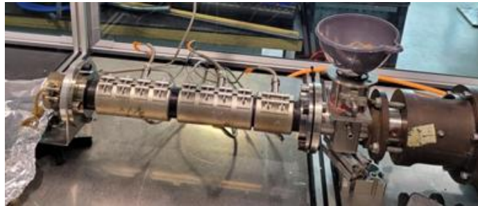
Figure 8: Extruder used in the process of biopolymer/wood fibres formulation.
