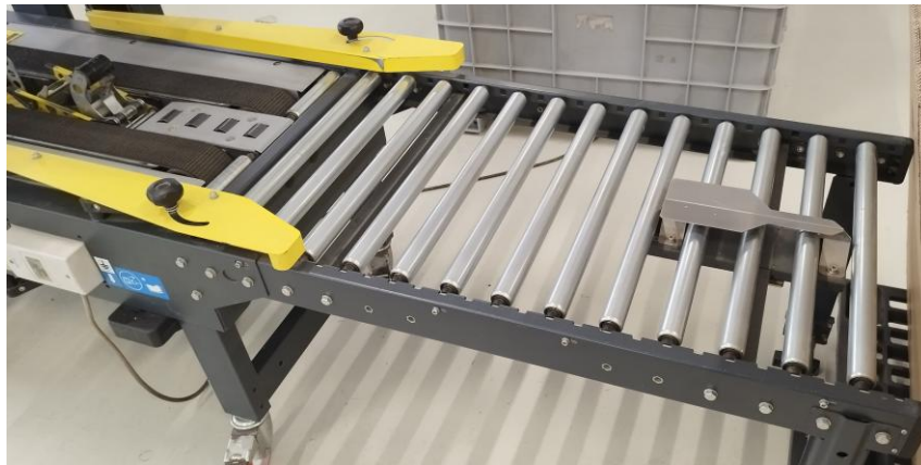
Figure 3: Conveyor roller in situ at LBRT.
