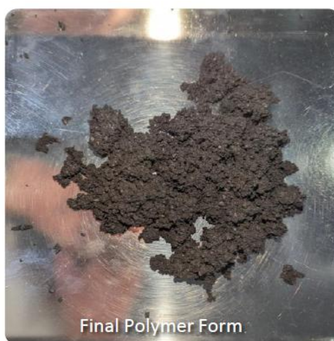
Figure 12: DES and ultrasound treated devulcanised rubber after compounding.
