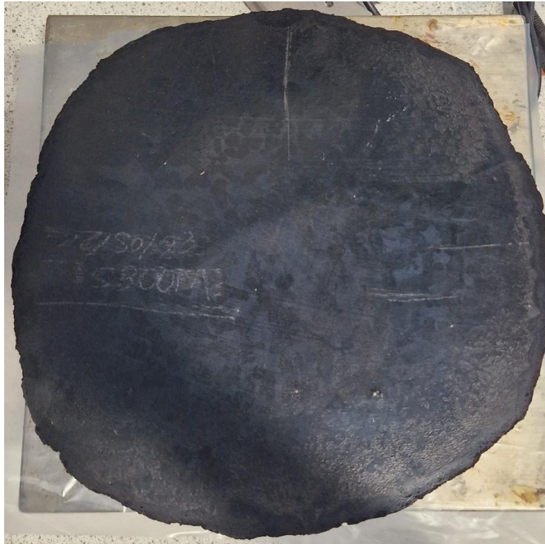
Figure 28: Panel removed at elevated temperature rather than colling under pressure. Pitting and blistering can be seen on the surface.
