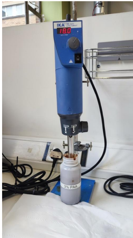
Figure 29: Mixing stage of the coating solution E, using IKA T25 digital Ultra Turrax at 18000 RPM
