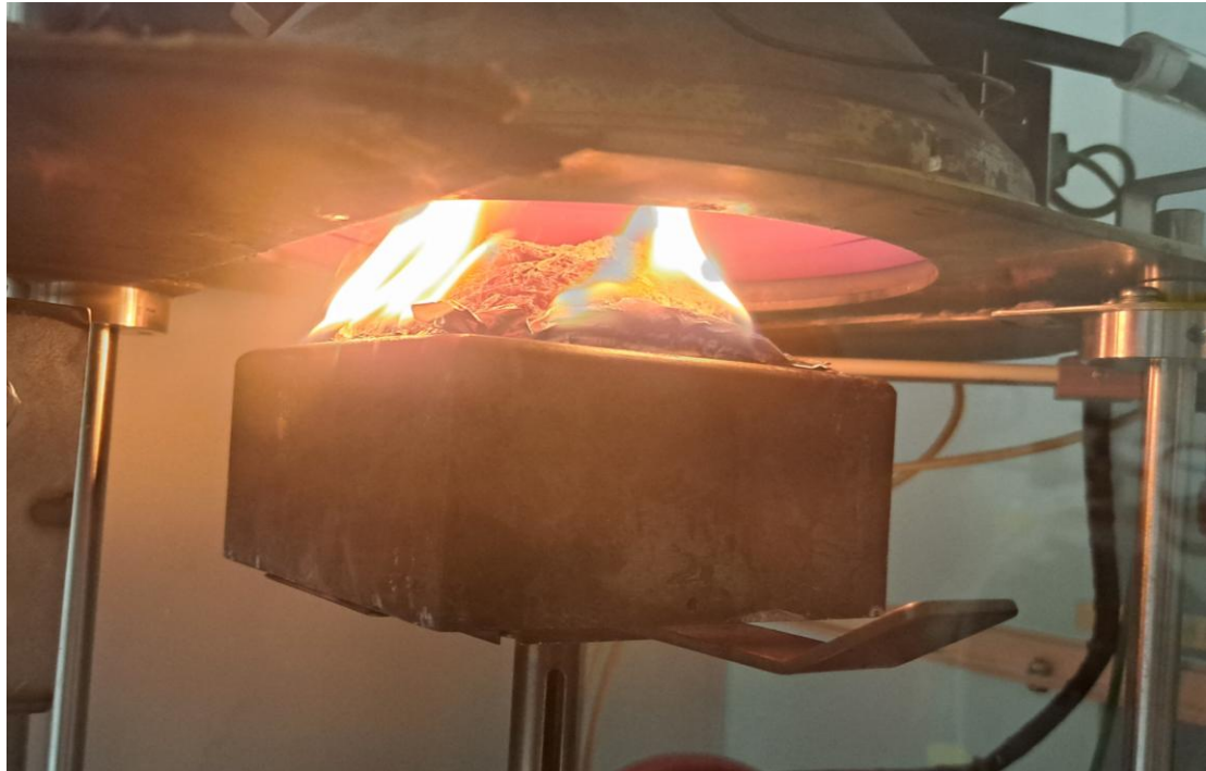
Figure 4: Extracted lignin during exposure on the cone calorimeter
