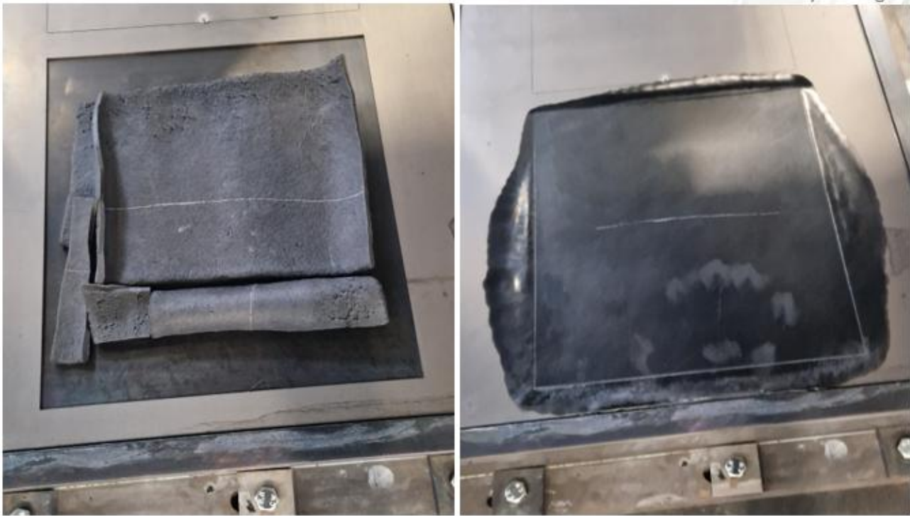
Figure 25: Left, rubber blank loaded into mould cavity before pressing. Right, rubber panel after pressing.
