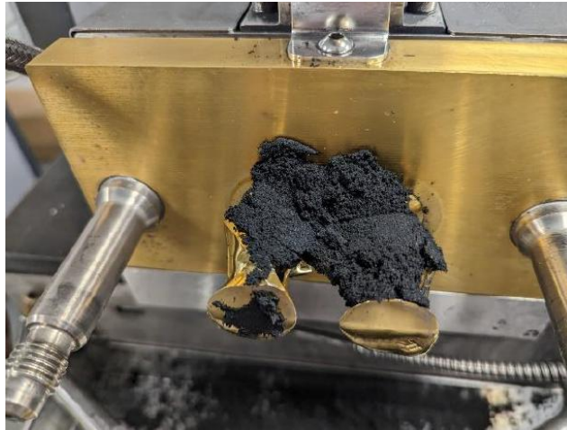
Figure 13: Crumb material remaining on the rotors of the internal mixer after the compounding process. Individual particles of rubber can still be seen.
