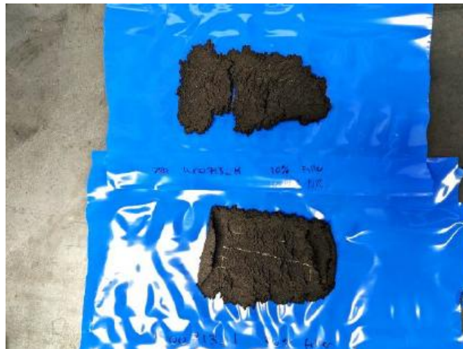
Figure 14: Top, devulcanised rubber with 10phr virgin natural rubber after compounding. Bottom, devulcanised rubber with 20phr virgin natural rubber after compounding.
