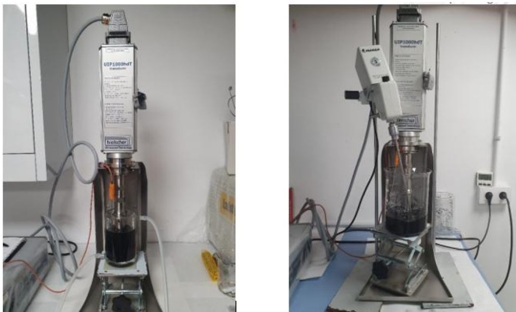
Figure 11: Ultrasound Prototype 1 for Chemical Devulcanization of Rubber using PO (left) and DES (right).
