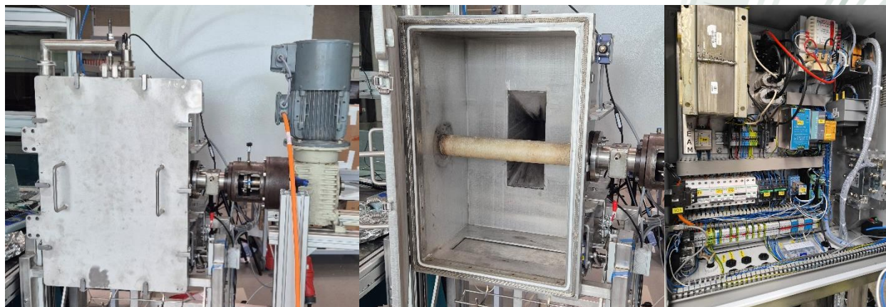
Figure 5. Whole WP5 MW setup, including the MW cavity with the screw motor (left), the open MW cavity with the specialised MW-transparent barrel (middle), and the inside of the control box (right).
