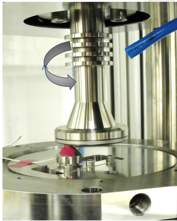
Figure 3: Tribological test rig (TRM 1000, Wazau, Germany) and test setup.
